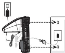
4. Align the holes on the bracket with the standard wall plate and slide the bracket down until it locks securely. Bundle the telephone line cord and power adapter cord neatly with twist ties.
