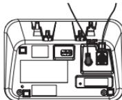
2. Position the telephone base against the wall mount bracket as shown. Insert the extended tabs marked **B** on the wall mount bracket into the slots marked **B** on the back of the telephone base. Push the telephone base down until it clicks securely.
